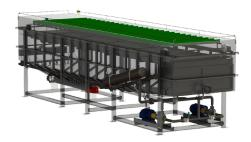
FRC's PWL-Series DAF handles heavy solids with a counter-current skimmer, large flotation surface, and sludge dewatering grid for efficient solids removal.
