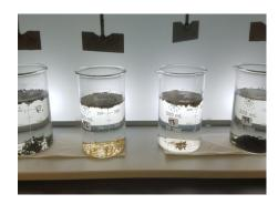
FRC performs jar tests to determine optimal coagulant/polymer dosing, simulate DAF performance, and reduce chemical costs.
